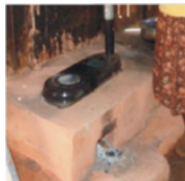
2-pot Chimney clay stove: built using Envirofit Z insert (2,000 ksh) and 2 pot chimney attachment (1,200 ksh): labor est. 400 ksh
